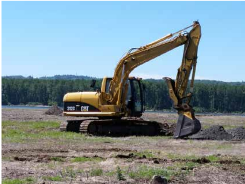
Photo 1. Caterpillar 312C excavator with ¼-yard bucket used for excavating. The view is towards the west-southwest.
