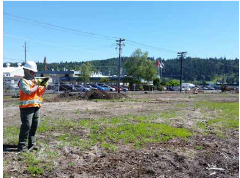
Photo 2. Trimble Geo XT in use to map geospatial test pit. The view is towards the northeast.
