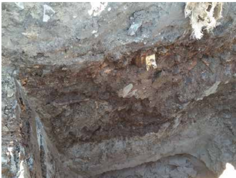
Photo 7. Profile of test pit TP-5 with presence of wood debris. The view is towards the west.
