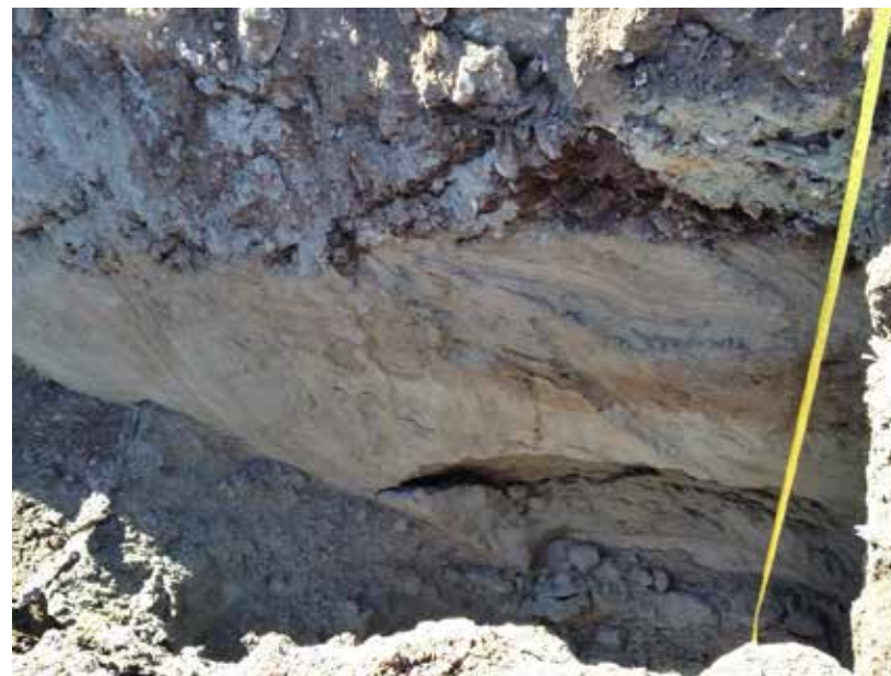
Photo 6. Profile of test pit TP-7 to a depth of 3.2 m (10.5 ft). The view is towards the south.
